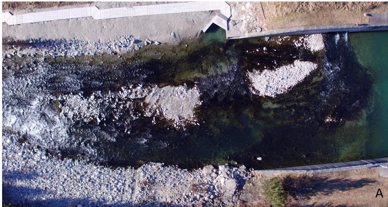
Figure 11. Capturing flow data from 3 different heights. A: height 75m, both banks in the frame; B. height 50m, banks only partially seen, fish ladder entrance not captured; C. height 25m, outflow from the turbine outside of the frame
